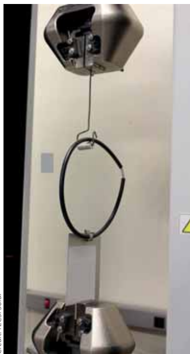
Figure 6. Wire clip mechanical load test
